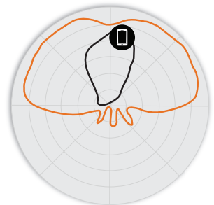
Figure 5 - T310d 5GHz Elevation Antenna Patterns
